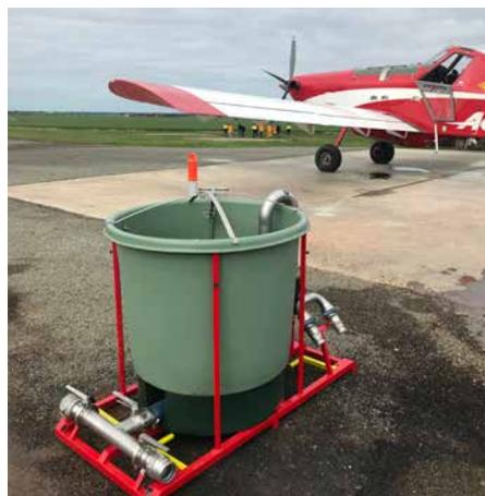
This plant is designed to supplement existing mobile or fixed airbase infrastructure used for the loading of Class A foam or water enhancers.
