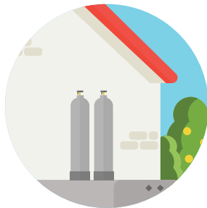
Position gas cylinders on side of house and away from trees and gardens
